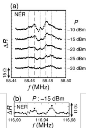
**Fig. 2** (a) RF power ( $P$ ) dependence of NER spectra taken near  $^{75}\text{As}$   $f_L$ . (b) NER spectra at  $2f_L$  for  $P = -15$  dBm. The NER signal was taken at  $\nu = 2$ . The dynamic nuclear polarization and detection were carried out by using  $\nu = 1$  quantum Hall breakdown.
