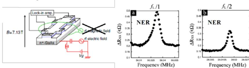
**Fig. 1** In the NER experiment, a sinusoidal rf voltage is applied to the backgate through a bias-tee after dynamic nuclear spin polarization. (a) and (b) show the NER signal at  $f_L$  and  $f_L/2$ . The NER was carried out at  $\nu = 2/3$  spin phase transition. The dynamic nuclear polarization and detection were also done by using  $\nu = 2/3$  spin phase transition.
